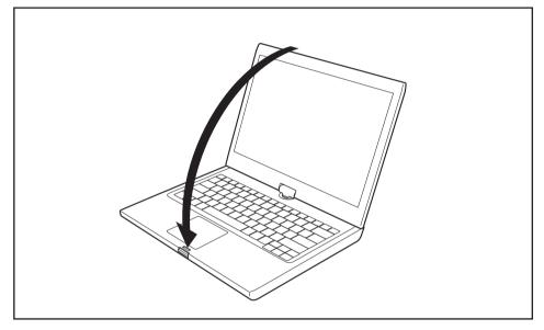
► Fold the LCD screen down onto the lower part of the notebook until you feel it lock into place.
